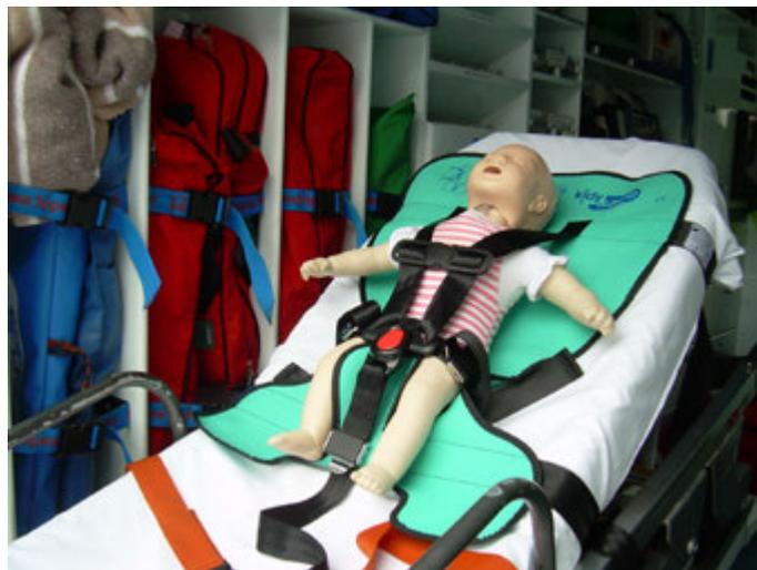
The device consists of a main canvas body with two adjustable straps to attach it to an ambulance stretcher and additional straps for restraining the child. These straps have a central fastening system and a quick release button.
